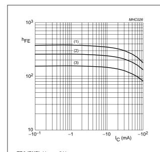
TR2 (PNP);  $V_{CE} = -5 \text{ V}.$
